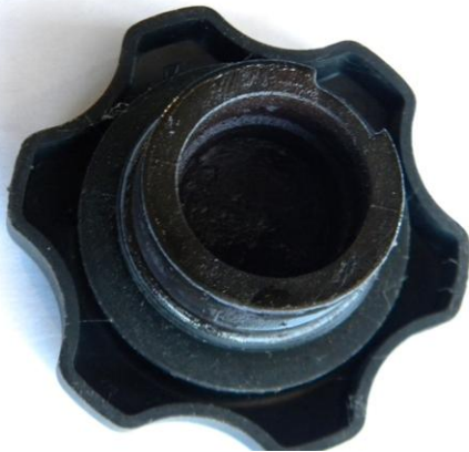
Photo 5 – Oil Fill Cap
