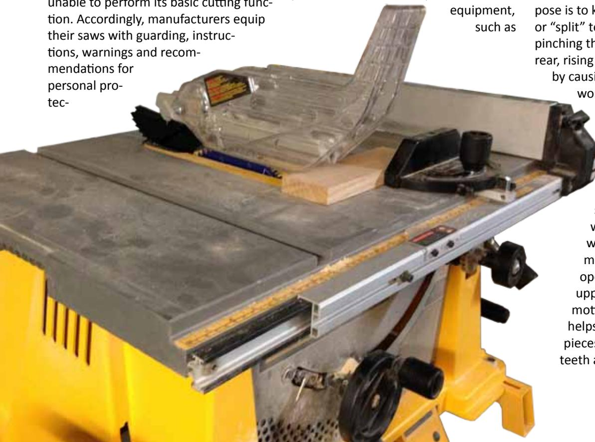
Example of a modern guard assembly with plastic barrier and anti-kickback pawls mounted on a riving knife.
